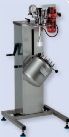
kiloclave with bmd 250 «i» and ATEX drive Glass lined steel vessels 1.0 – 20 liter Pressure max. 12 bar, max. 200°C Components and internals made of PTFE, PFA, glass lined or Tantalum
